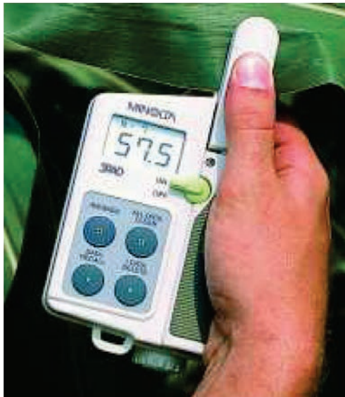
Figure G-6. Handheld chlorophyll meter used to monitor nitrogen status of corn plants.
