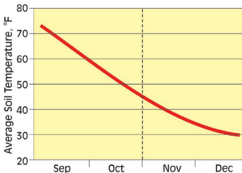
Figure G-4. Average soil temperature in the fall at Clay Center, NE.
