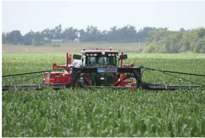
Figure G-7. Onboard plant chlorophyll sensors used to adjust nitrogen fertilizer application.
