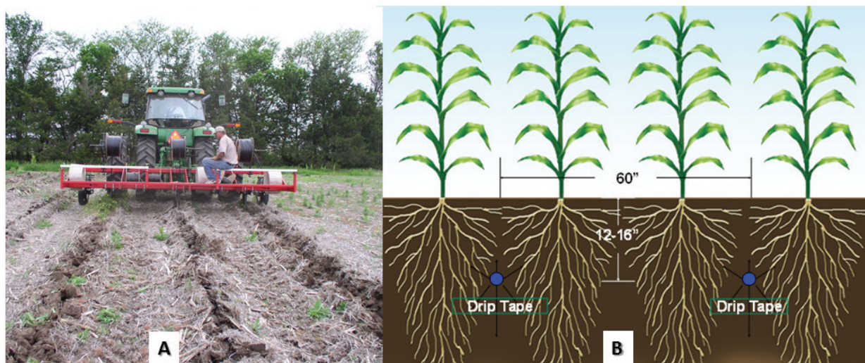
Figure M-1. Diagram showing a cross-section of a cornfield with SDI drip tape installed to provide equal access to water by each corn row.
