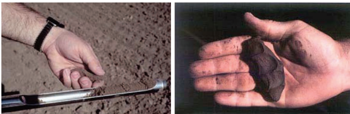
Figure J-3. Sampling and evaluation techniques for the feel method of soil water monitoring.
