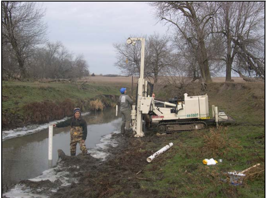
Dr. Xunhong Chen and Dr. Mark Burbach, both of the University of Nebraska-Lincoln, conducted streambed conductivity tests on the West Fork Big Blue River. Streambed conductivity data was needed for the Blue Basin Groundwater Model. Eighteen sites were tested in the Blue River Basin.
