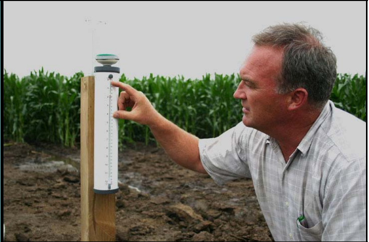
Pictured above, Dan Leininger, NRD Water Conservationist, takes a reading from an atmometer, which simulates the evapo-transpiration of a corn leaf.
