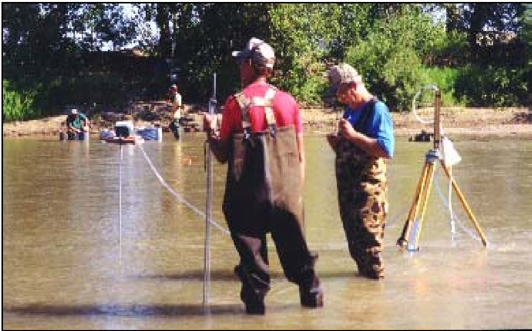
Stream gauges are calibrated with depth and velocity measurements to determine flow rates. This picture was taken near Lewellen, Nebraska, upstream of Lake McConaughy.
