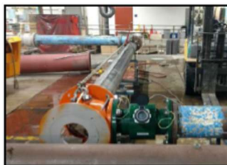
Zero Distance from Turbine Pump Discharge
