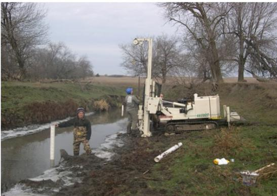
*Dr. Xunhong Chen (left) and Dr. Mark Burbach, both of the University of Nebraska-Lincoln, conducted streambed conductance tests on the West Fork-Big Blue River. The drilling and testing was to find out how fast water moves vertically through the streambeds.*
