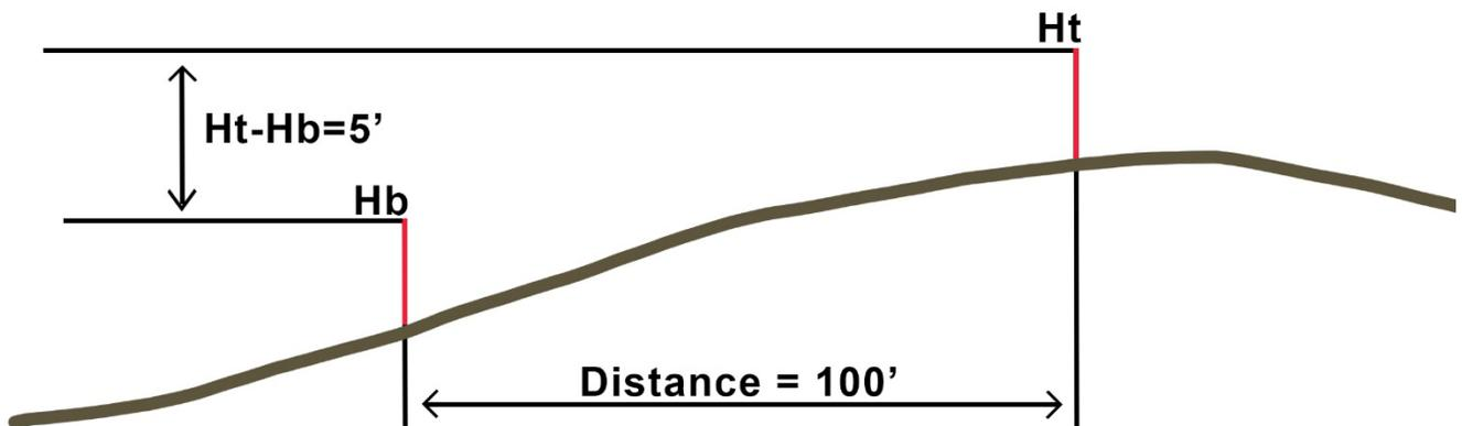
At 100 foot spacing of stakes the difference in the elevation of the stakes equals the percentage of the slope. In this case the slope would be 5%.
