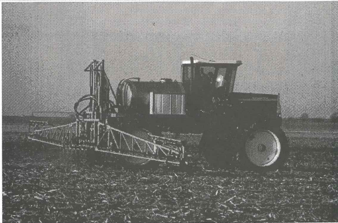
Figure 1. Applicator used to apply UAN solution with Agrotain.
