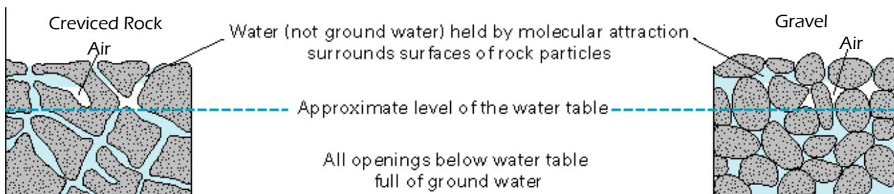
**Figure 1.** Basic aquifer concepts (U.S. Geological Survey).
