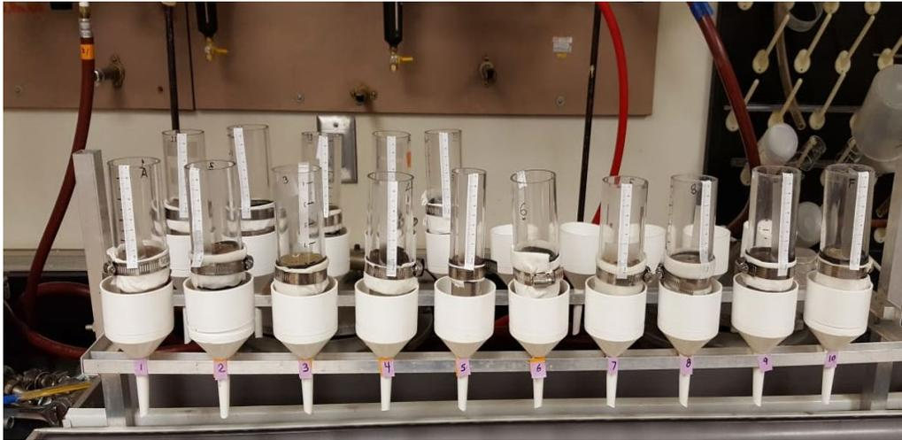
**Figure S1:** Falling head setup with soil core
