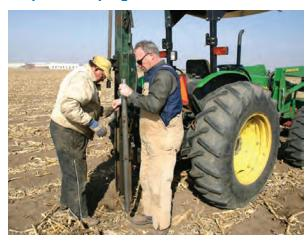
As part of the groundwater regulations, the Upper Big Blue NRD personnel perform deep soil sampling at each of the nine monitoring well sites every five years. The purpose is to collect data regarding nitrate levels in the soil, as well as the direction and speed the leaching nitrates are traveling.
